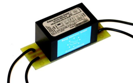
Protective module of Bajog electronic GmbH (litz wire version)
