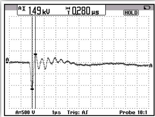
The voltage load (depending on location and on grid characteristics) can be measured between 1 - 10KV/µs.
